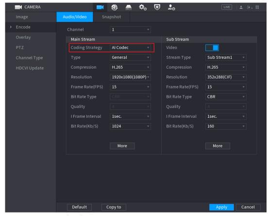
ii. Configure the settings for the main/sub streams parameters.
